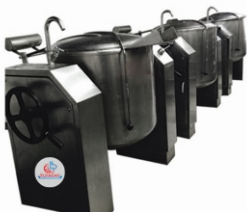
Vessel Gearbox system
